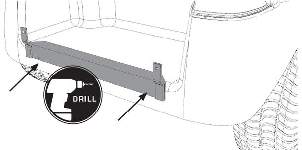
Remove Bumper Angle from car and attach to footrest supports.
