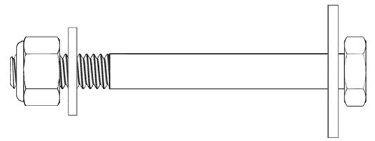
1/4" X 2-1/2" Hex Bolt - 1/4" Fender Washer - 1/4" Flat Washer - 1/4" Nyloc Nut
