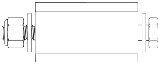
1/4" X 2-1/2" Hex Bolt - 1/4" Flat Washer (x2) - Spacer Square - 1/4" Nyloc Nut
